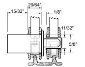
Spring activated plunger allows locking without key on all plunger locks.
